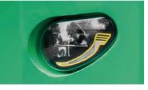
The whole vehicle is equipped with LED, and the integrated headlamps have daytime running lamps, far/near light, front turning streamer and other functions.
